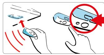
Sensor faces towards you. Make sure that the Heat Sensor is fitted tightly on to the mounting plate.
