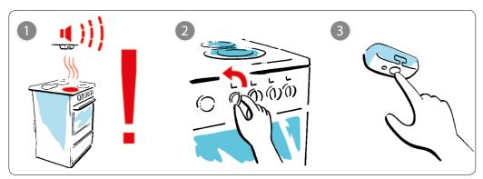
If the Stove Guard has turned the cooker off, first turn all cooker knobs to '0', then press the Heat Sensor cover once. (In cookers that are operated by touch, just press the Sensor cover once.) After this the cooker can be used normally.
