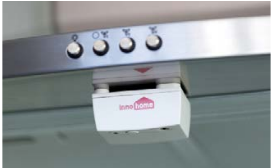
The intelligent heat sensor in the Stove Guard and in Stove Alarm follows the heat but in addition also tracks the rate of increasing temperature
