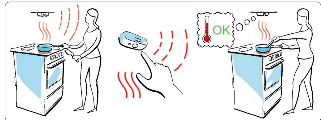
Pressing the Intelligent Heat Sensor cover during the pre-alarm signal (
