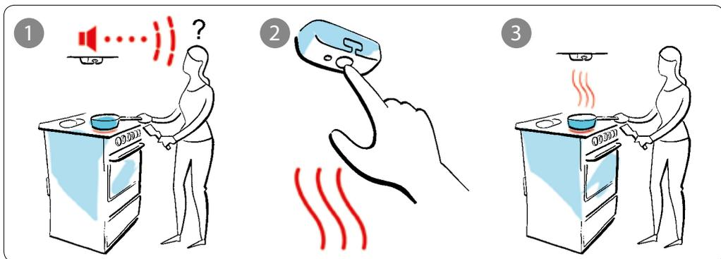
If the Stove Guard starts to signal during cooking, press the Heat Sensor cover once.
