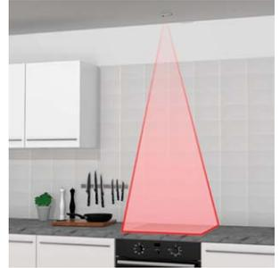
For ceiling installations, the supplied IR lens extension must also be fitted. See page 10.
