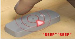
3. An unadjusted Sensor's sensitivity setting is level 8, and when checking the level, the Sensor gives a set of "beeps" as follows: 8 - 8 - 5 - 8. If the sensitivity was adjusted to level 4, the sensor would give "beeps": 4 - 4 - 5 - 4.
