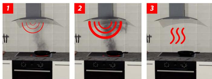
**1.** The Stove Guard sounds a pre-alarm in case of potentially dangerous situation while cooking. **2.** If the warning is not acknowledged, the stove guard alarms and cuts off the power to the cooker. **3.** When the cooker has cooled down to a safe temperature, it is ready to be used again. Just press the sensor button once.
